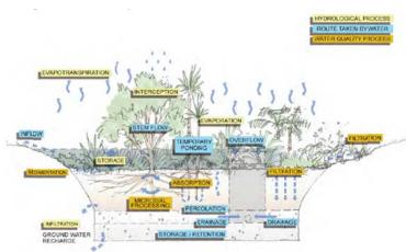
Forested bioretention cell schematics. .This project will employ internal water storage to increase nitrogen reduction through increased denitrification with increased residence time, decreased outflow water volume, and decreased temperatures of water flows to the receiving streams.
